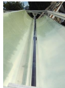
Figure 10 The receiver tube.
