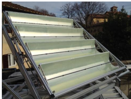
Figure 9 The small size parabolic collector.
