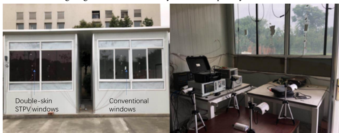
Fig 1. Test rig and measurement instruments
