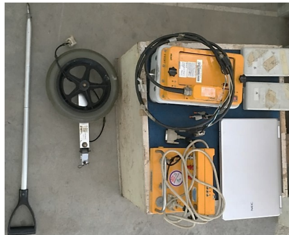
Figure 2. The GPR equipment set for frequency 800 MHz.
