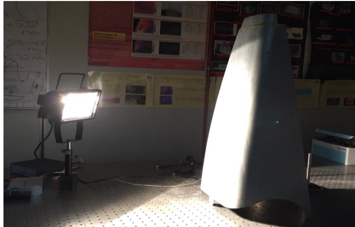
Figure 6. Arrangement of 500Watts infrared spotlight during heating of A320 Aft Fixed Fairing sample
