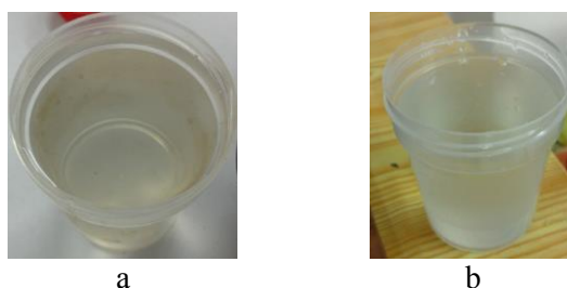
Figure 8. The liquid after some stages of treatment: a – n = 300 \div 320 rpm, b – n = 110 \div 240 rpm.
