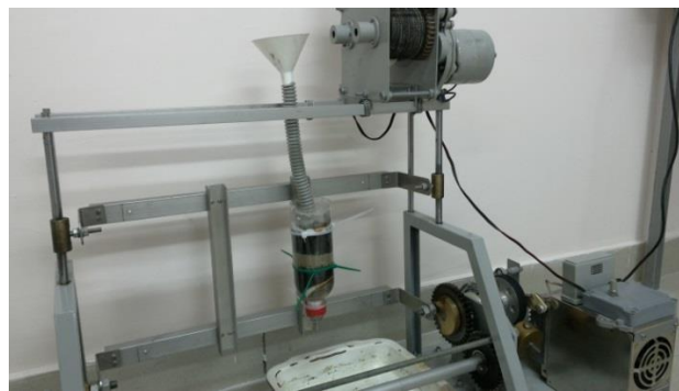
Figure 5. An experimental plant of a vibration and centrifugal unit with a filtration chamber vertically installed.
