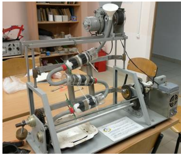
Figure 6. An experimental vibration and centrifugal plant for treatment of liquids.
