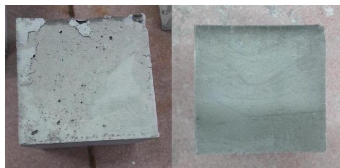
Figure 2: Surface of Portland cement concrete (left) and geopolymer concrete (right) after artificial seawater exposure
