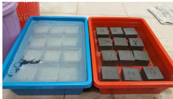
Figure 1: Sample observation 7 days after exposure to artificial seawater
