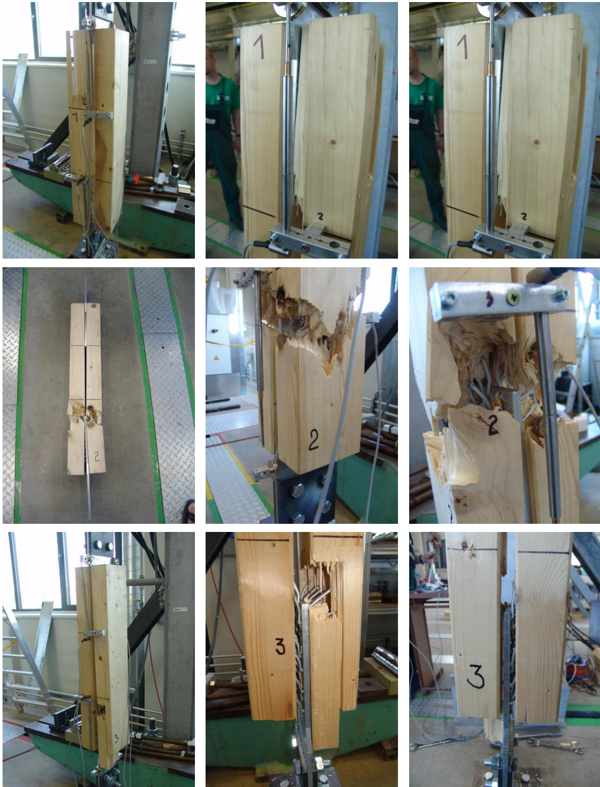
Figure 5. Damaged specimens – overall view and important details of the specimens V1 (1st row), V2 (2nd row) and V3 (3rd row).
