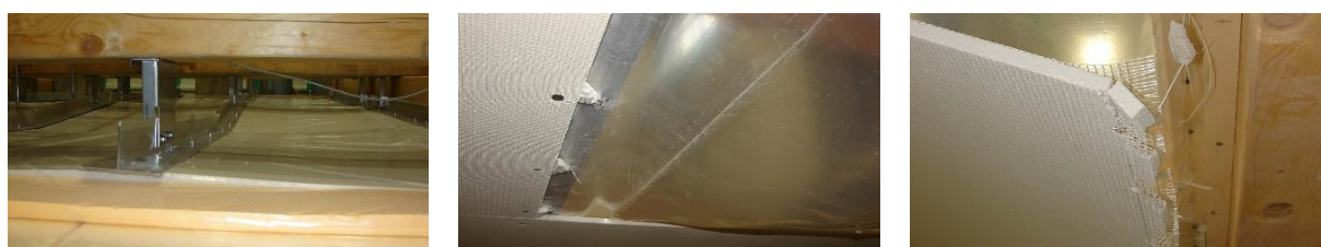
Figure 6. Examples of specimen failures recorded during vacuum testpmpg – T-profile buckling of specimen 1 (left), cladding elements failure at a fixing of specimen 1 (middle) and cladding elements failure at a fixing of specimen 6 (right).
