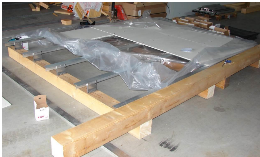
Figure 2. Preparation of the facade system specimen (including the assembly wooden frame) intended for vacuum testing – aluminium subframe arrangement 1.
