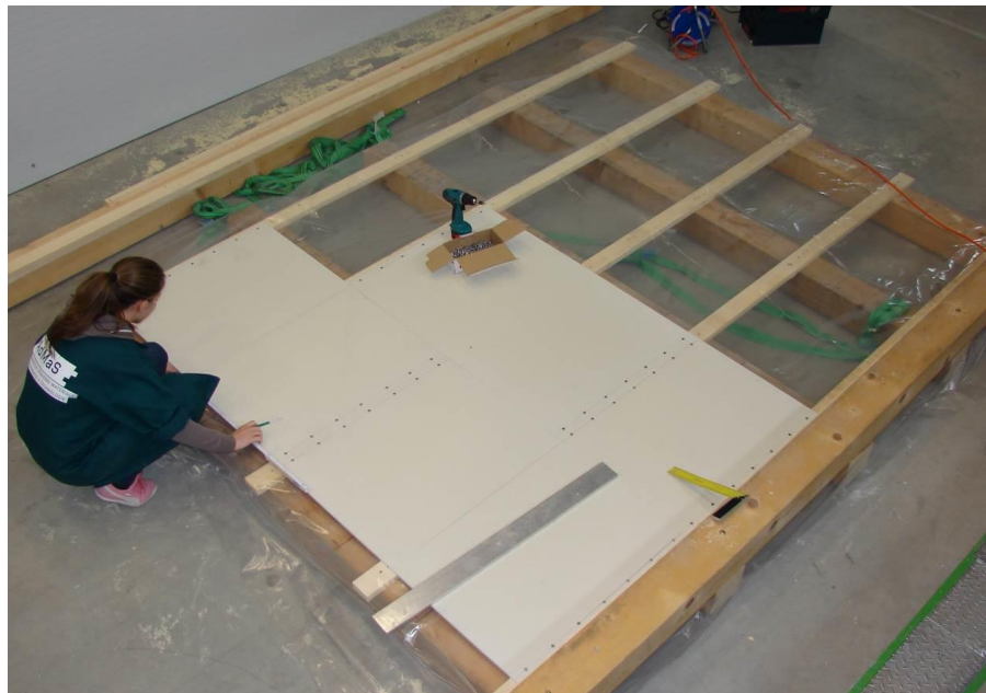
Figure 3. Preparation of the facade system specimen (including the assembly wooden frame) intended for vacuum testing – timber subframe arrangement 6.
