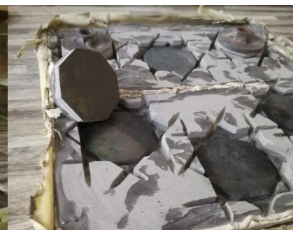
Figure 5. Place of failure after pull-off test in the contact zone grout/cast basalt surface.
