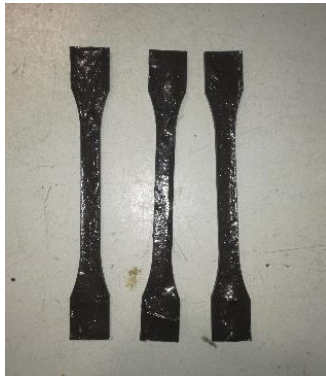
Figure 6. Specimens in the shape of dog bone for determination of tensile properties.
