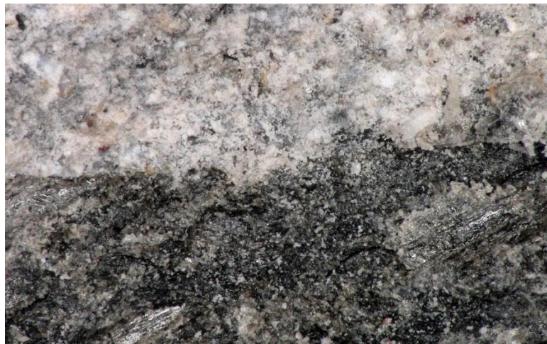
Figure 12. The connection detail of developed grout (30% TOS2) to cast basalt tile (magn. 64×).
