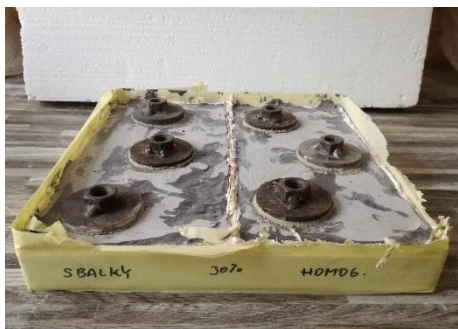
Figure 3. Metal targets glued for the determination of cohesion to cast basalt.
