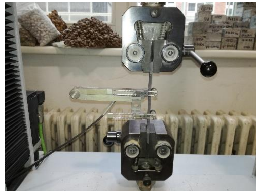
Figure 7. Loading test specimen of the polymer grout by a tensile force in the test device.
