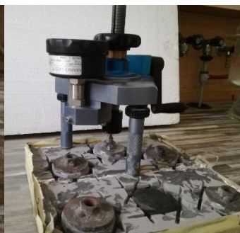
Figure 4. Performing the pull-off bond strength test.
