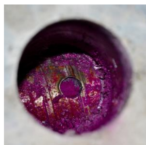
Figure 7. A drill to the steel protection pipe, breaking off the drill and puncturing the pipe to the cable. Currently, standard practice of checking.
