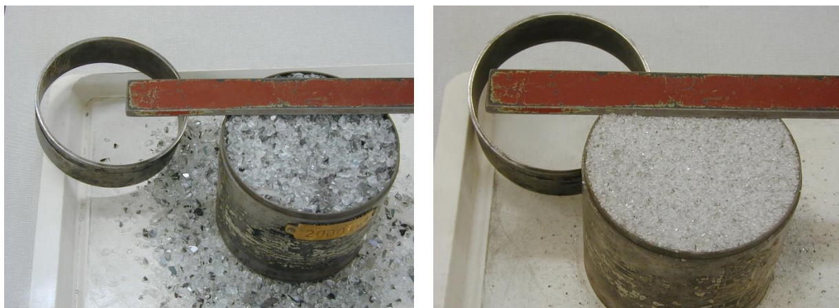
Figure 4. Determination of bulk density of glass recyclate of fractions of 4-8 mm and 1-2 mm.
