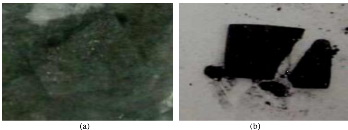
Figure 5. Brake pad composites damaged during friction test: (a) PR-10; (b) PR-15
