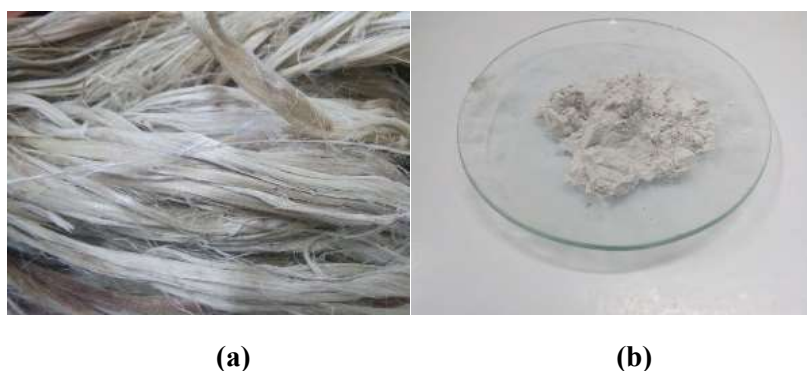
Figure 1. The image of (a) kenaf fiber, (b) calcium carbonate particle
