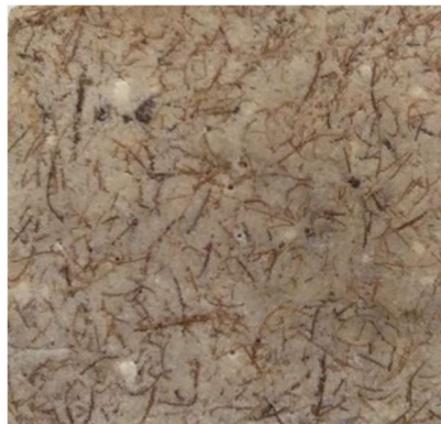
Figure 1. Composite specimen for brake pads material
