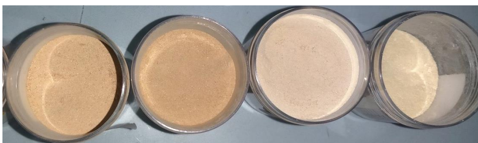
Figure 1. Chitin powder color comparison: A. Chitin from method A (single fermentation with L.plantarum ); B. Chitin from method B (single fermentation with B.thuringiensis ); C. Chitin from method C (co-fermentation with L.plantarum , continue with B.thuringiensis ); D. Chitin from method D (chemically extracted chitin).
