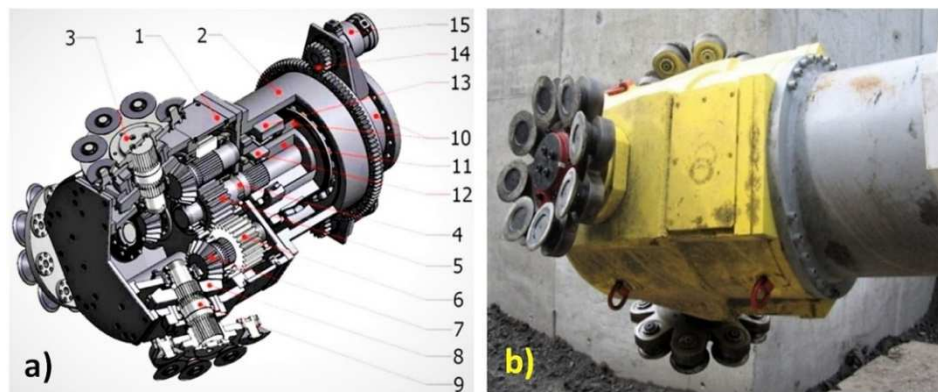
Figure 15. The new mining head solution with disc tool of complex trajectory: a) – spatial model, b) - view of KR150 roadheader mining head ready before field tests [11]. 1 – main gear, 2 – auxiliary gear, 3 – disc plate, 4 – input shaft, 5 – central gear wheel, 6 – orbital gear wheel, 7 – pinion, 8 – face gear, 9 – output shaft, 10 – support, 11 – connector, 12,13 – bearings, 14 – body gear, 15 – hydraulic engine.
