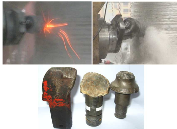
Figure 3. View of frictional sparking and dustiness during cutting of a rock sample with a rotary-tangential pick and wear of pick wedge.
