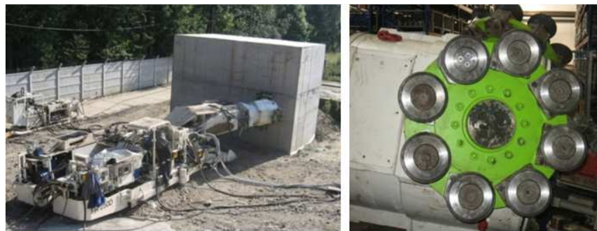
Figure 17. A view of FR250 roadheader with new mining head with disk tools before the field tests [13].
