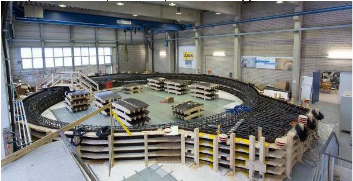
Figure 5. Laboratory testing of concrete reinforcement in the Thermal Energy Storage unit of ADELE project [6].
