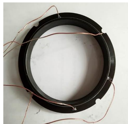
Figure 8b. The innstallation of thermocouple.
