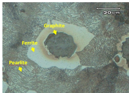
Figure 3. The microstructure of SG iron as-cast, nital 3% etchant.
