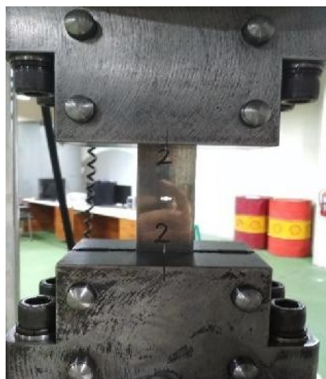
Figure 3. Fixture of dynamic test machine for specimen
