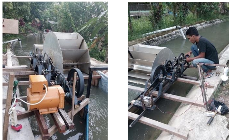
Figure 1. The arrangement of water wheel apparatus in irrigation
