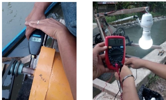
Figure 2. Rotations and Voltages measurement
