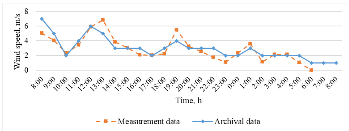
Figure 5. Graph of measurements of wind speed from SEN0170 sensor in comparison with archival data.
