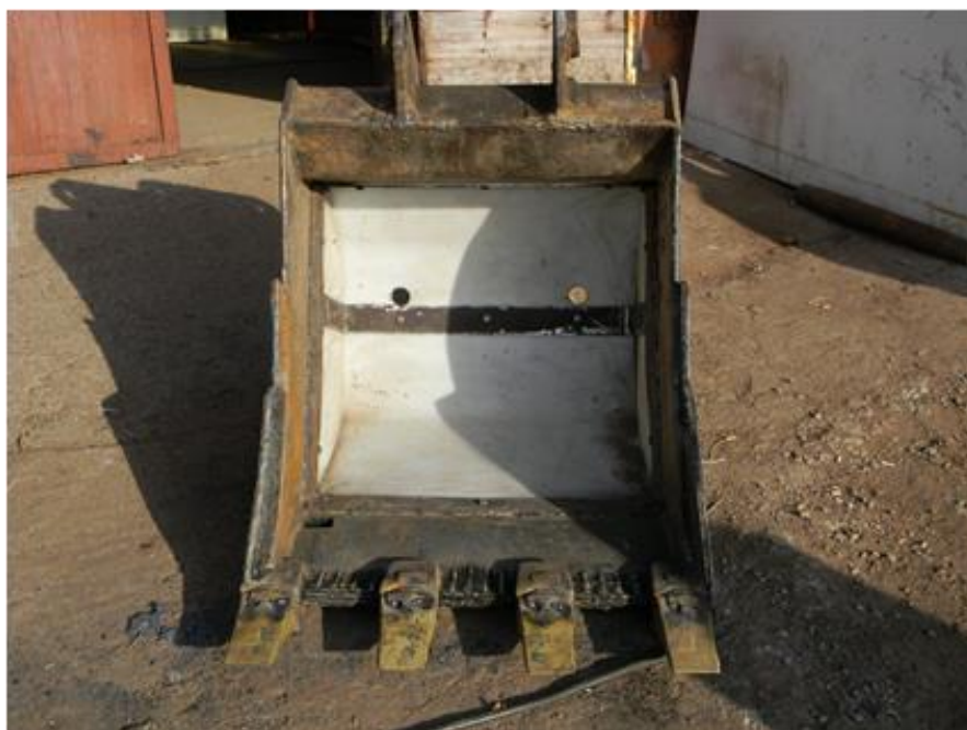
Figure 2. EK-18 excavator's bucket before operation.
