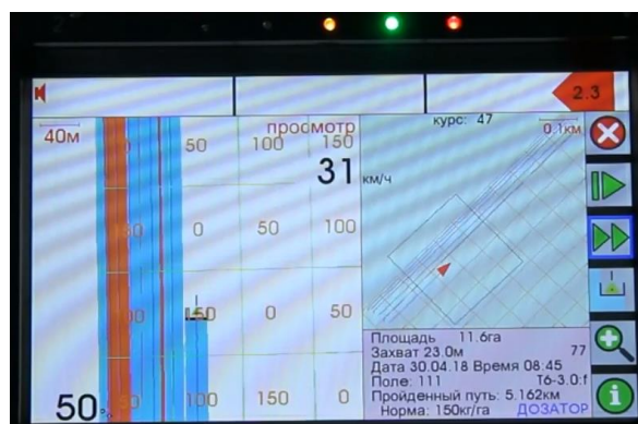
Figure 2. General view of the map for the differential fertilisation on the monitor of Agronavigator (in the Russian language).
