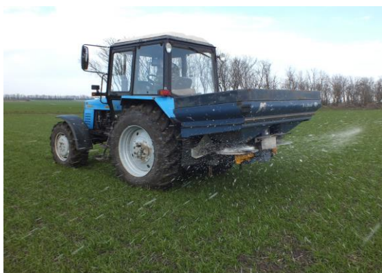
Figure 1. Bogballe M2 Spreader equipped with “Agronavigator-Asur-Dozator” system together with Belarus 1025.2 tractor.
