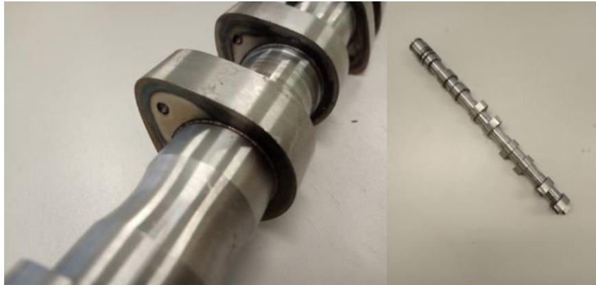
Figure 4. Camshaft after combined (preheating + weld) processing.
