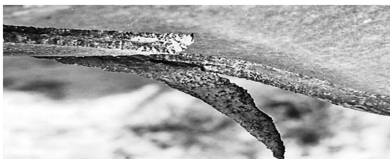
Figure 2. Disclosure of colony of cracks at destruction of the pipeline (X70 steel).
