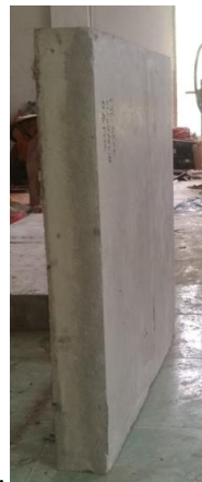
(b) The final result of foam concrete based macro-encapsulated PCM
