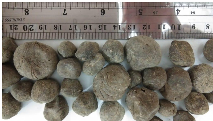
Figure 2. Macro-encapsulation PCM of beef tallow/damar gum.
