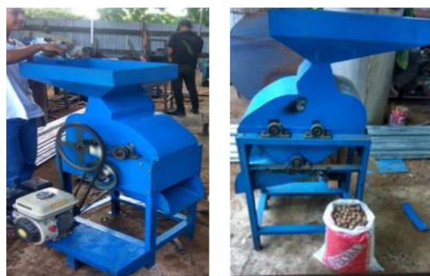
Figure 2. Assembled dried areca nut peeling machine
