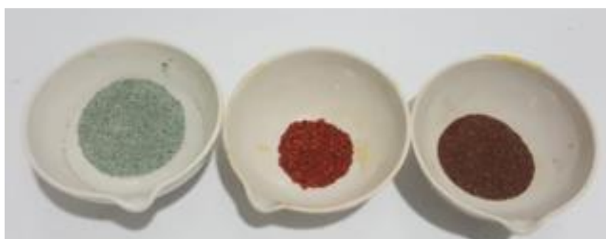
Fig. 1 (A) Natural Zeolite (B) Zeolite-FeO (C) Zeolite-FeO-Sucrose
