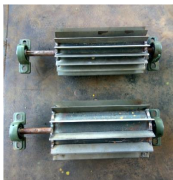
Figure 1. Cylindric cutter's blade in the drum
