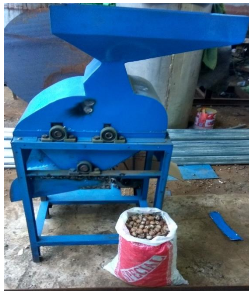
Figure 2. Construction of peeling-machine and peeled areca nuts
