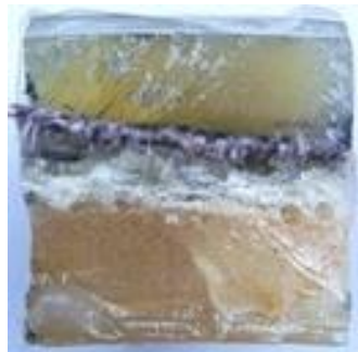
Figure 8. Fracture surface section from impact testing
