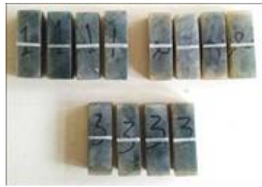
Figure 5. Hybrid composite impact test specimen
