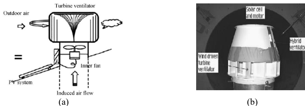
Figure 4. Hybrid PV-Wind Powered Turbine Ventilator (a) Illustrative diagram of the prototype device developed in [3], (b) Full-scale model developed in [5]
