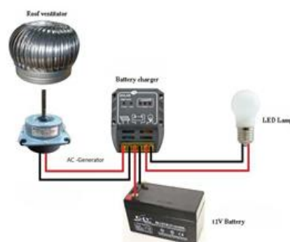
Figure 5. The main components of system electric power generation by RTV
