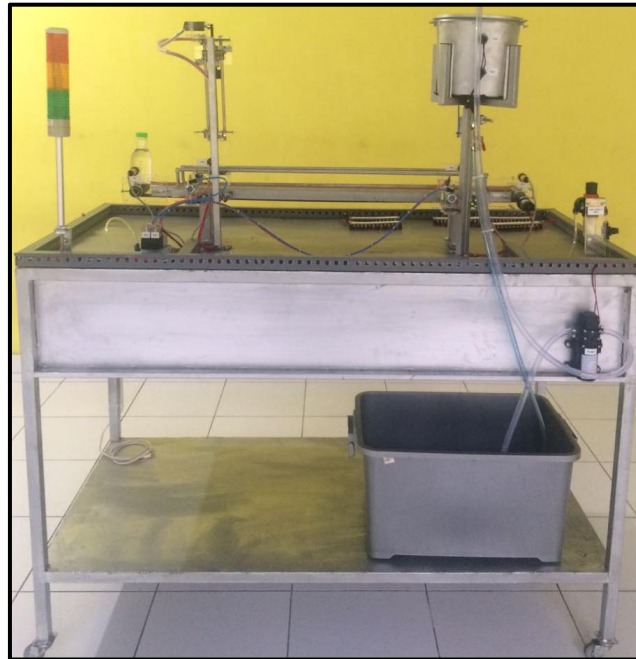
Figure 1. Automatic water filling and capping machine trainer kit prototype as PLC practical learning trainer kit for vocational high school.
