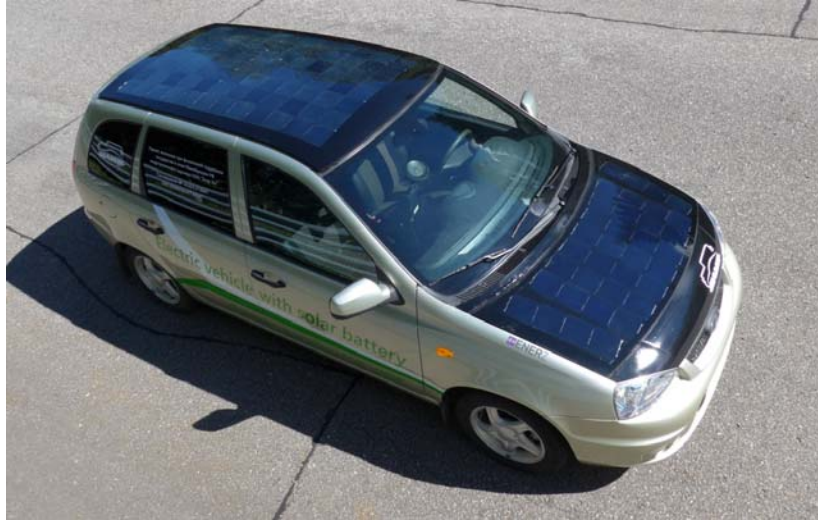
Figure 2. General view of an experimental electric vehicle with PV, developed and manufactured in the FSUE "NAMI".
