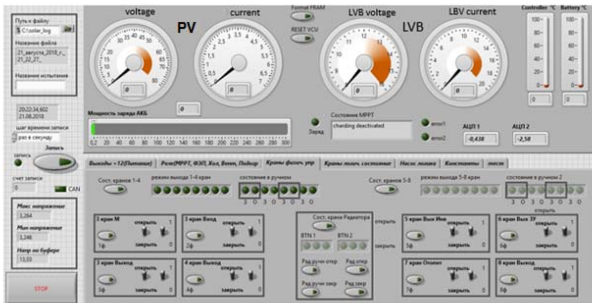
Figure 9. The system for indicators of electric vehicle with a PV system monitoring.
