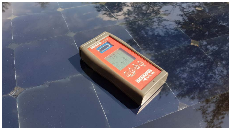
Figure 11. Measuring of the solar energy intensity.
