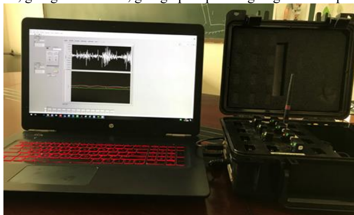
Figure 1. Acquisition of the sEMG singals and ACC signal.
