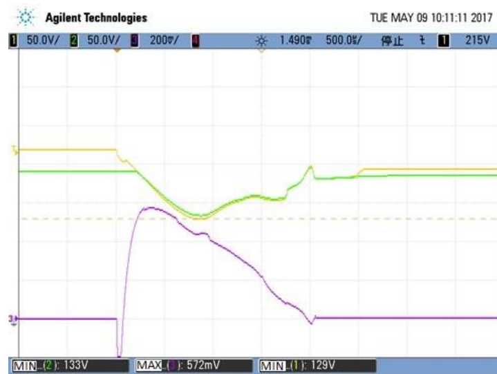
Figure 7. Short circuit test waveform of feeder lines for 16 12V batteries in series and 16 parallel battery modules running simultaneously (1mV is corresponding 4A).
