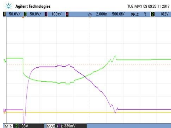
Figure 6. Short circuit test waveform of feeder lines for 16 batteries in series (1mV is corresponding 4A).
