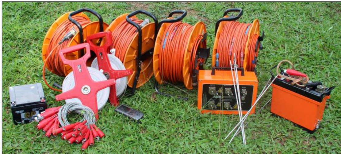
Figure 3. ERI Survey equipment
