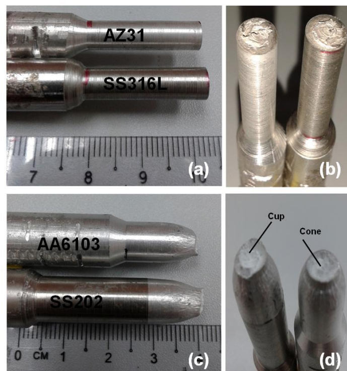
Figure 4. (a-b) The macro photographs of the tensile tested and the ductile fracture surface of tensile tested specimen AZ31/SS316L. (c-d) The macro photographs of the tensile tested and the brittle fracture surface of tensile tested specimen AA6103/SS202.
