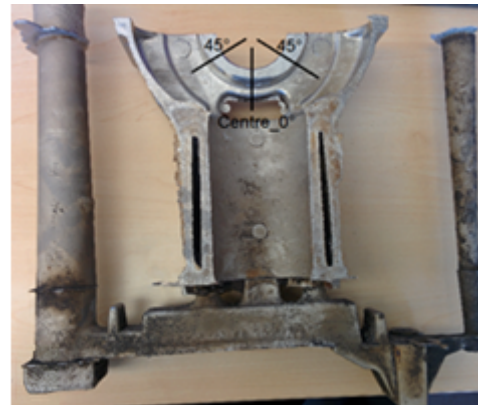
Figure 2. Cast engine block section – the lines show the approximate locations where metallography samples were taken
