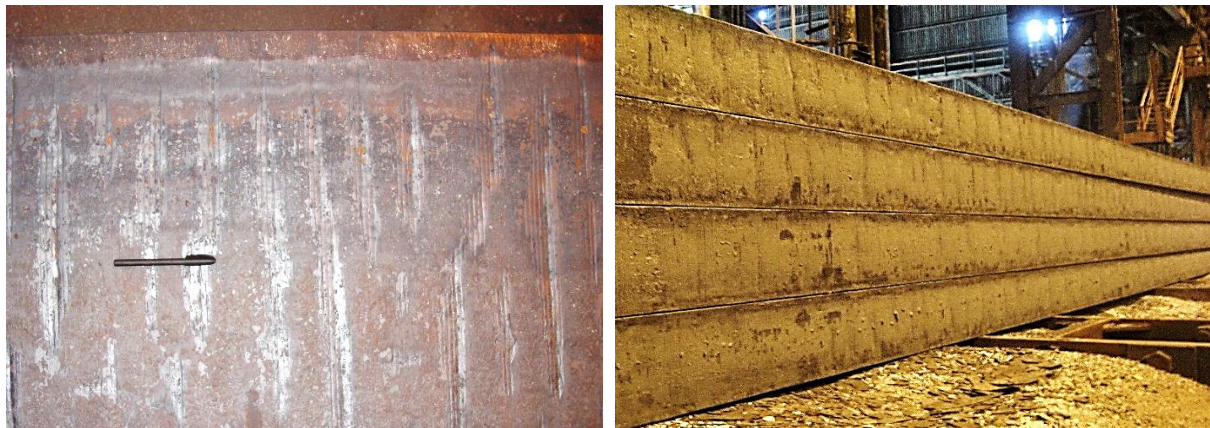
Fig.5 Transverse depression on as-cast AHSS slab surface at an equal spacing (Left – BF and Right – NF).
