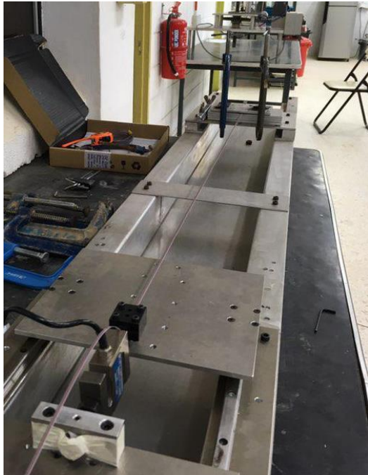
Figure 4a. Fibre optic tensile load test.
