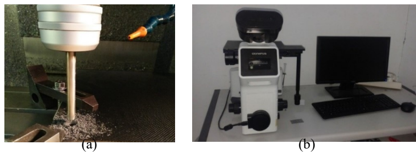
Figure 1. Setup of the experiment (a) drilling process (b) tool wears measurement process.
