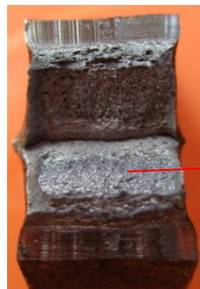
Figure 11. The fracture surface of the base metal.
