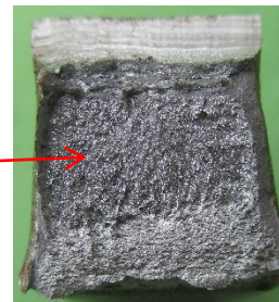
Figure 11. The fracture surface of the base metal.
