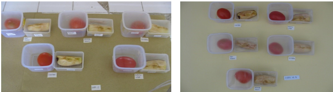
Figure 2. Visual illustration of the testing process as bioplastic packaging pieces of apples and tomatoes (Left: first day and Right: after seven days)
