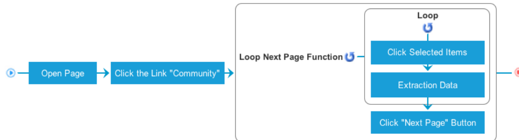
Figure 3. Logical schematic diagram of GooSeeker's main grabbing technology route.
