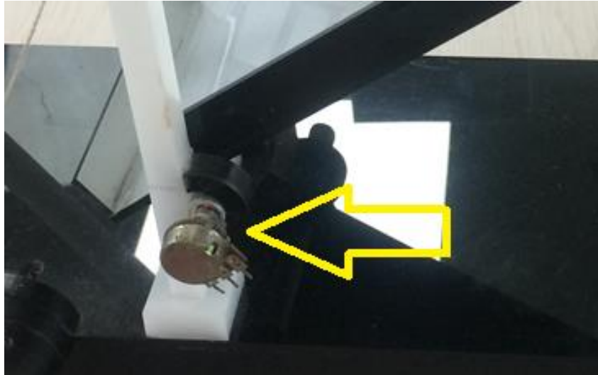
Figure 8. Potentiometer coupled to the axis of the platform.
