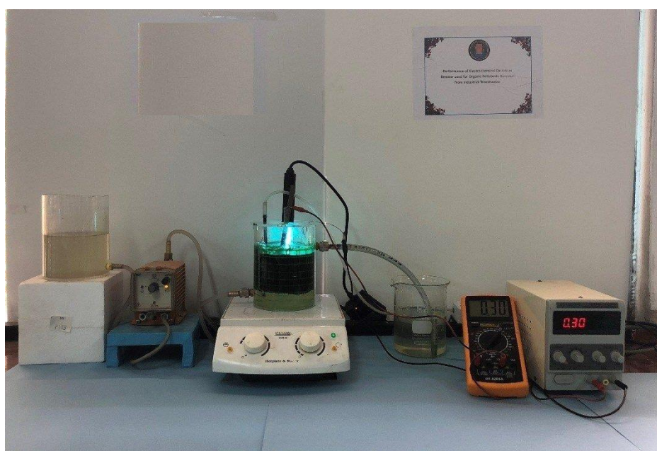
Figure 2. Photograph of continuous photoelectron-Fenton experimental system.
