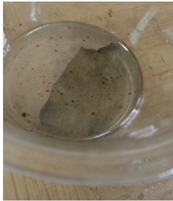
Figure 1. carbonate slices dipped in Nano fluid
