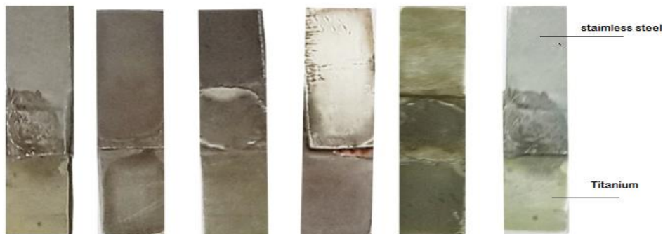
Figure 2. diffusion bonded lap joints
