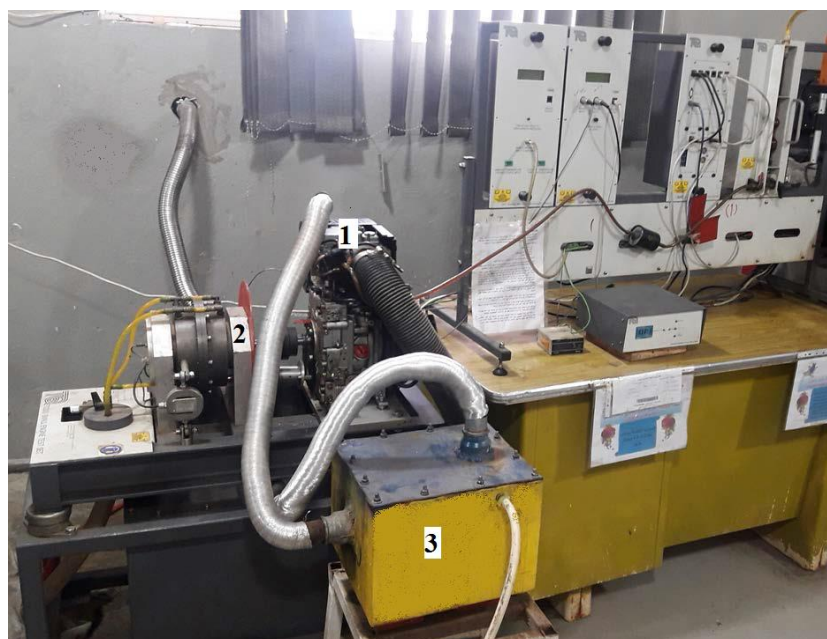
Figure 3. Test set-up: 1- diesel engine, 2- hydraulic dynamometer, 3- water bath.
