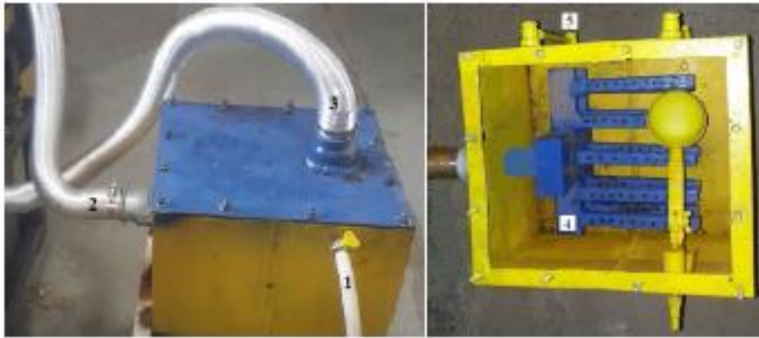
Figure 2. Water bath; 1- water inlet, 2- exhaust gas inlet, 3- exhaust gas exit, 4- perforated tubes, 5- water outlet.
